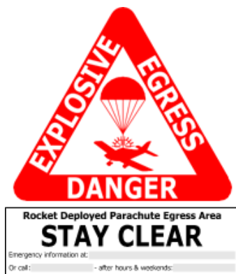
Figure 2 - Sample label with danger placard. Danger placard to be dimensioned in as defined in Figure
