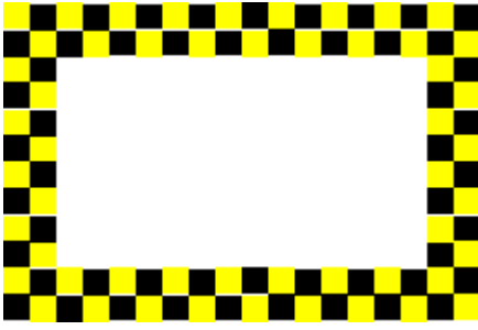
Figure 3 - Sample marking of stored energy device exit area
