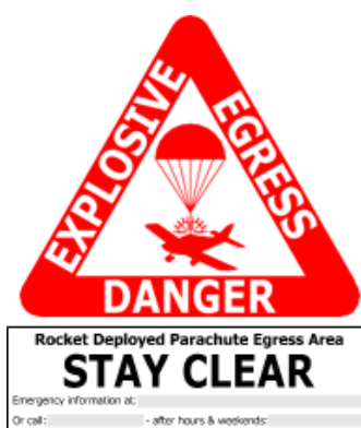
Figure 2 - Sample label with danger placard. Danger placard to be dimensioned in as defined in Figure 1
